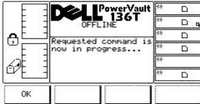
Figure 54. Command > Drives > Unload > Dialogue Command in Progress
